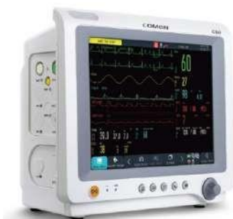
DALC80 Multi-parameter Patient Monitor 12.1" LCD touch screen
